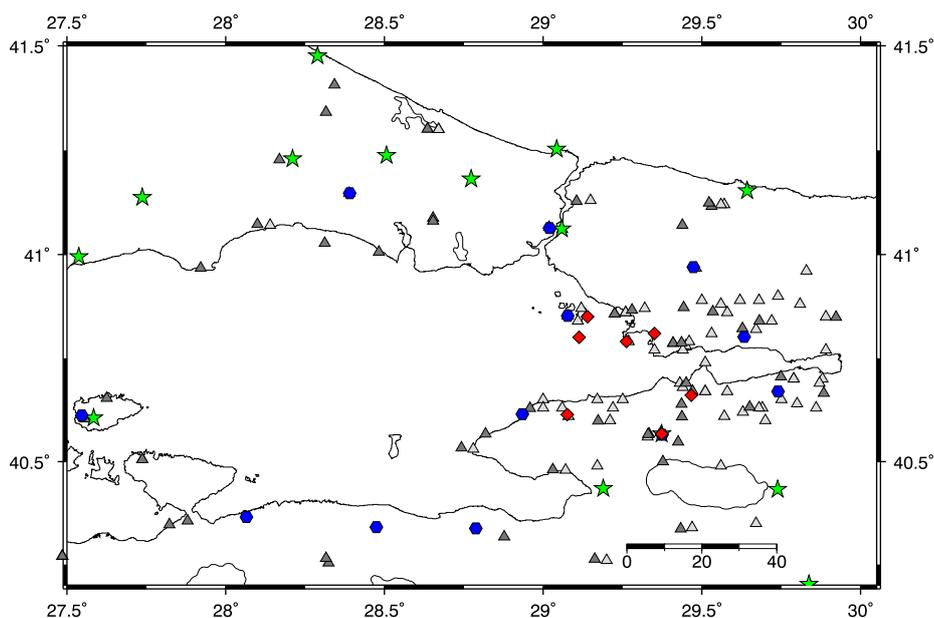
**Fig. 2.** Map of seismic stations in the eastern Marmara region. Gray triangles show the locations of the stations operated after 17 August 1999 Izmit Earthquake. Red diamonds are CINNET stations installed in 2008. Blue hexagons correspond to temporary IPGS stations installed before the Izmit earthquake. Green stars are the locations of the permanent KOERI stations installed between 2006 and 2008.
