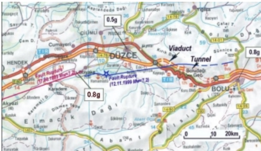
Figure 9. Peak horizontal ground accelerations recorded in the Duzce earthquake
