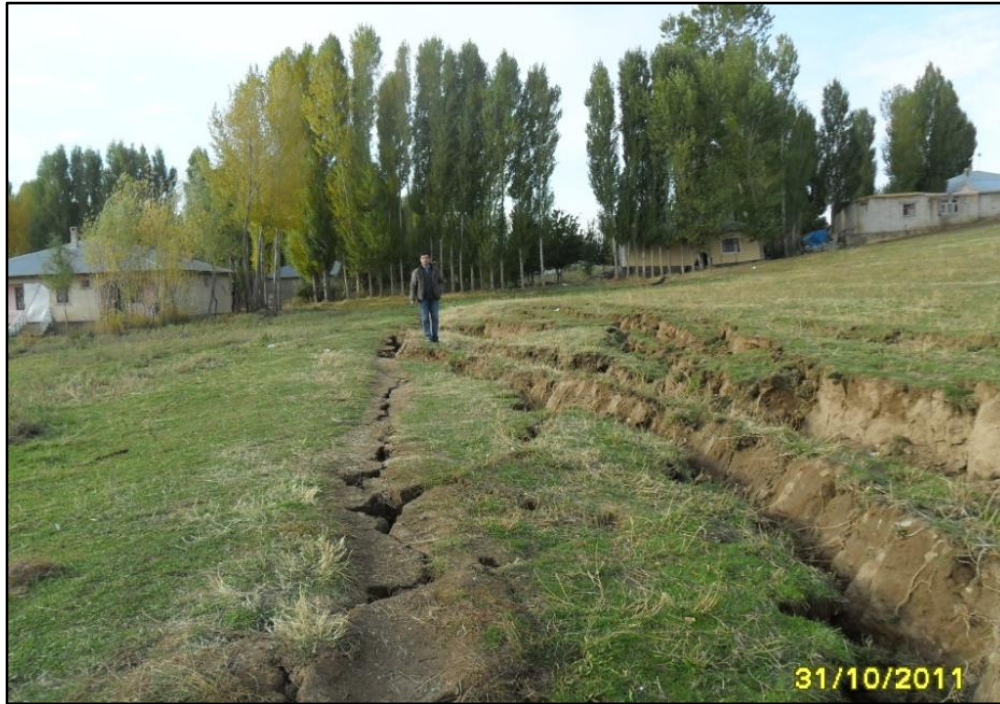
Figure 23. Soil cracks due to land slide in Celebibag, Ercis
