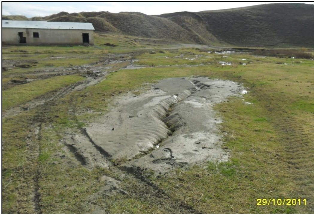
Figure 25. Sand boils due to liquefaction in Topakca (Mermit) village, Van
